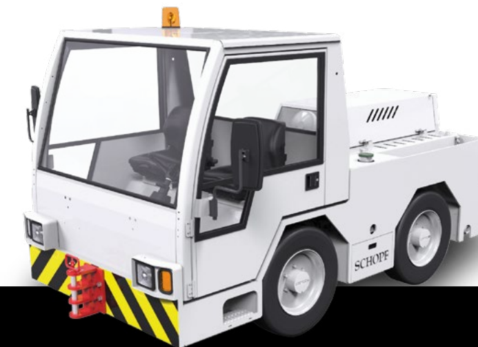
F59 10,116 lbf | 10,790 lbf | MTOW ≤ 154,000 lbs IIIA | EU STAGE V US EPA Tier 3 | US EPA Tier 4F
