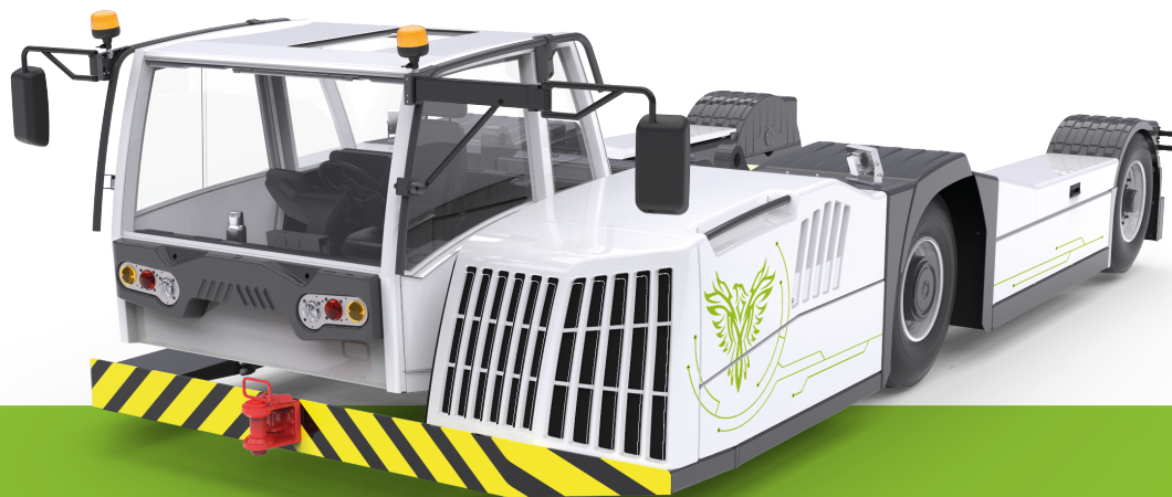
»PHOENIX« AST-2E 70 kWh | 140 kWh | 210 kWh 20 mph | MTOW ≤ 776,000 lbs
