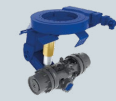
+ Goldhofer driven pendular axle with ball bearing race ring, hydraulic worm gear drive and electronic steering
